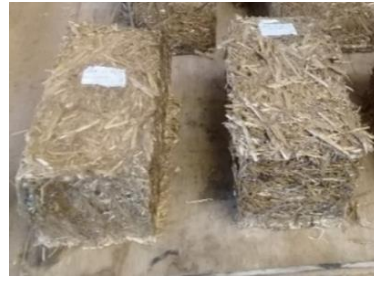
b) Block type 2 made of chopped straw mixed with Binder
