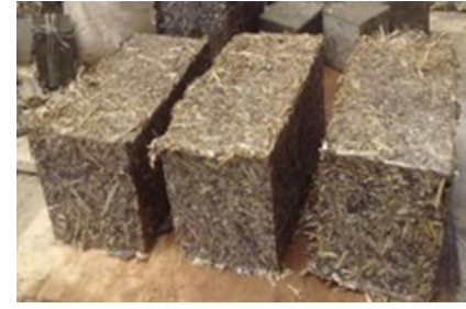
c) Block type 3 made of chopped straw mixed with saw dust and binder
