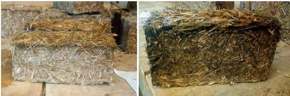
Fig. (8). Failure pattern after the Initial Rate of Absorption test.
