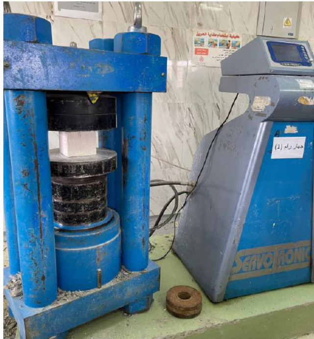
Fig. (4). The sample of AAC under the compressive strength test.
