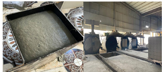
Fig. (3). The green cake in the mold and the autoclave of AAC.
