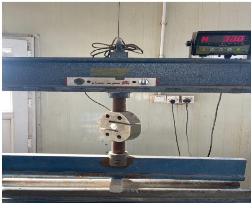
Fig. (6). The sample of AAC under the flexural strength test.
